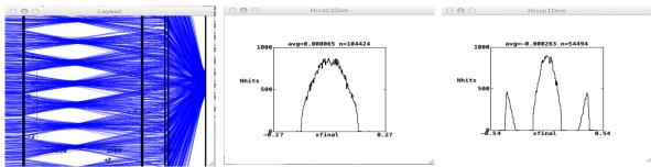
Another good reason for using an illumination array is that joint areas in the imaging MLA may be geometrically ill-defined, and can make spurious contributions to the final intensity distribution; for e.g if they were small planar sections this would lead to an axial hot spot of the resulting parallel rays being focussed by the Fourier lens.
