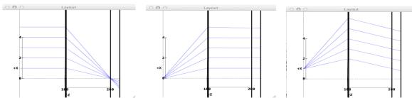
Thus, two lenses can image a point source or sources, where lateral distances are multiplied by the ratio of the lens focal lengths, giving rise to the notion of magnification. Note this occurs independently of inter-lens separation, but if in addition the latter is equal to the sum of the focal lengths then initial ray directions are also preserved (inverted), as is most obvious by examining initially parallel rays (at right). Such an arrangement of lenses is termed an optical relay.
