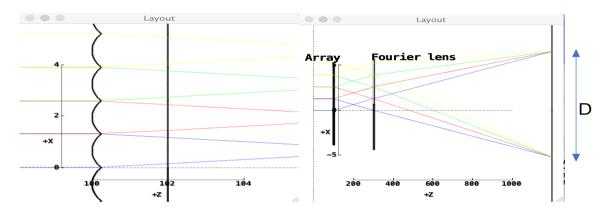
The width of the final distribution **D** is equal to  $\mathbf{p} \times \mathbf{Ff}/\mathbf{Fa}$ , where  $\mathbf{p}$  is the **array pitch** (i.e. microlens size) and **Ff** & **Fa** are the focal lengths of the Fourier lens and MLA respectively. However, this simple explanation hides some complexity...
