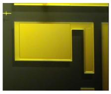
Using a lighter gas atmosphere is the next best option, and He the only practical safe solution, providing reasonably effective debris control. The photo at left indicates opening of contact areas to gold film; the width of the larger opened area here is approx. 1mm. Just a trace of redeposit can be seen between this zone and its neighbour above(out of the picture).
